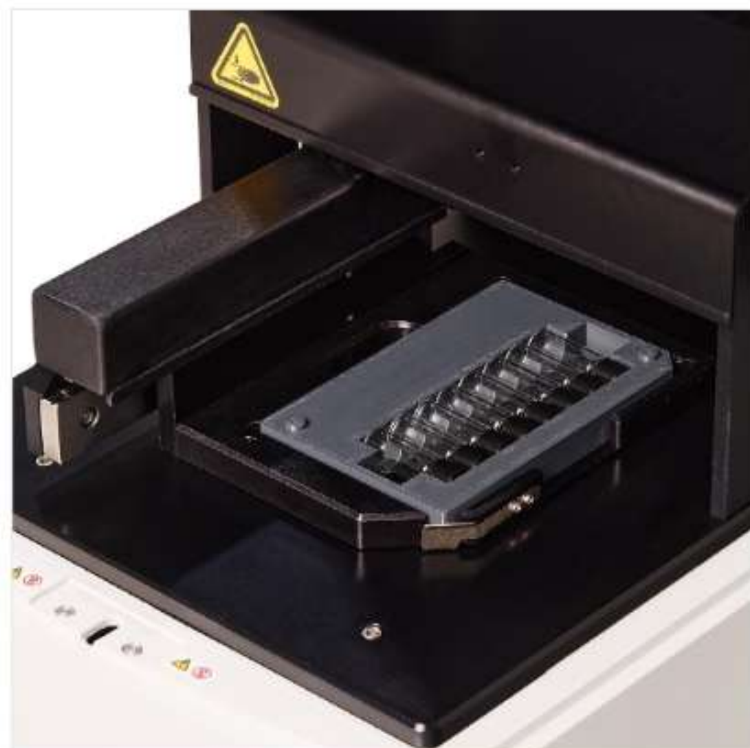
User-created 8-vial holder loaded into the Automatic Sampling Array (ASA) accessory.
