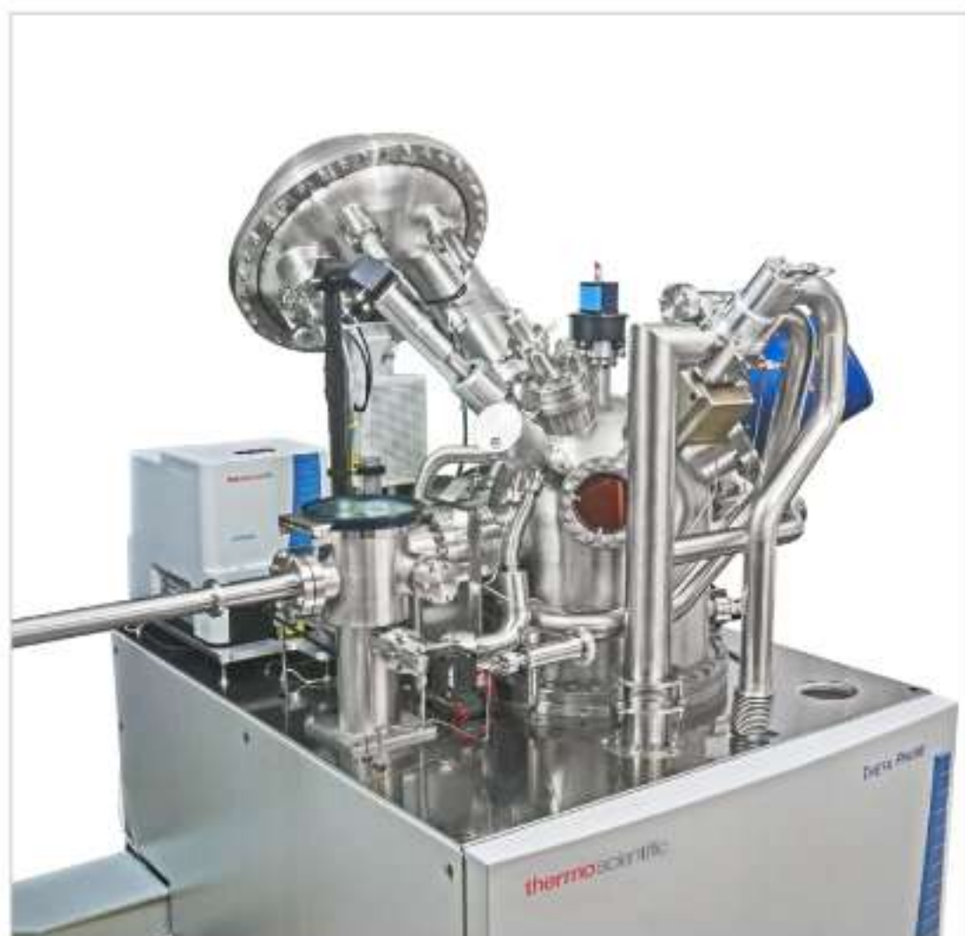
DXR3 Flex Raman Spectrometer coupled with a Thermo Scientific Theta Probe XPS Spectrometer.
