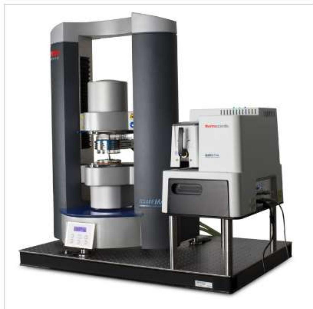
DXR3 Flex Raman Spectrometer coupled with a Thermo Scientific HAAKE™ MARS™ Rheometer.
