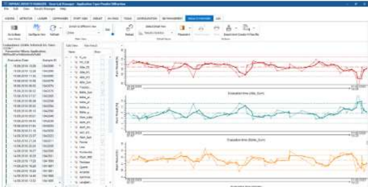
Figure 2 Results manager view, showing selected results of TOPAS quantitative phase analysis results from a cement plant.
