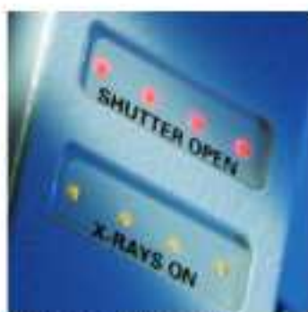
X-ray tube LED status display
