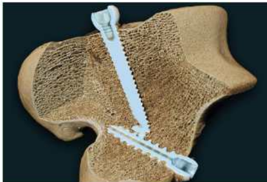
Sheep bone 60 mm in size with 2 titanium implants, 5 mm in diameter.
